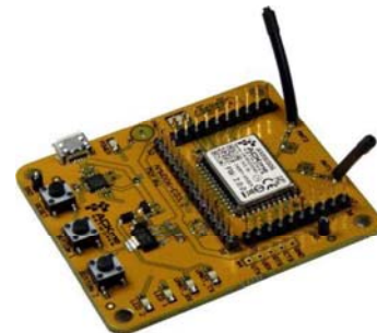
Figure 9 - AMW006-E03 eval board with wire antennas
